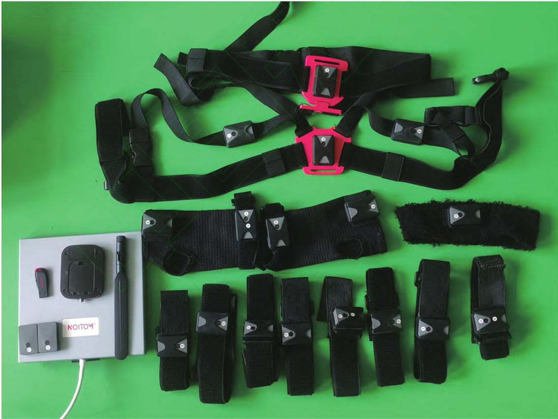
图2 Noitom Perception Legacy动作捕捉设备 Figure 2 Motion capture device of Noitom Perception Legacy
